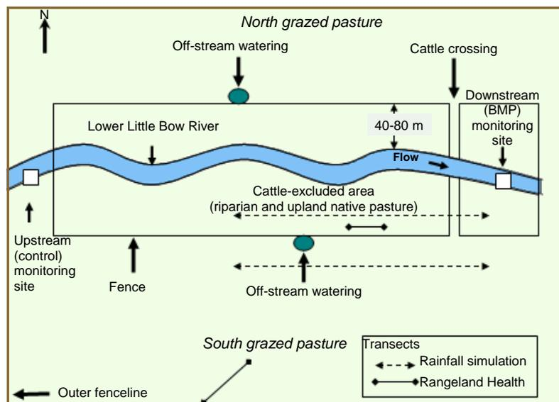
Figure 2. Schematic diagram of streambank fencing with cattle crossing
