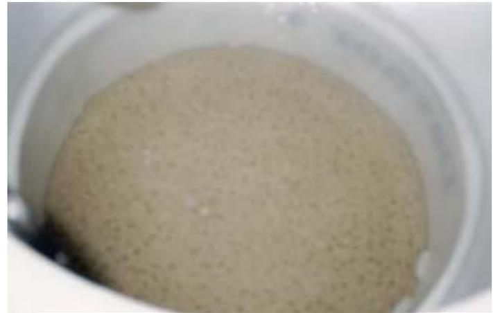
The biological layer developed on top of sand (2 cm) may require replacement to remove accumulated surface deposits
