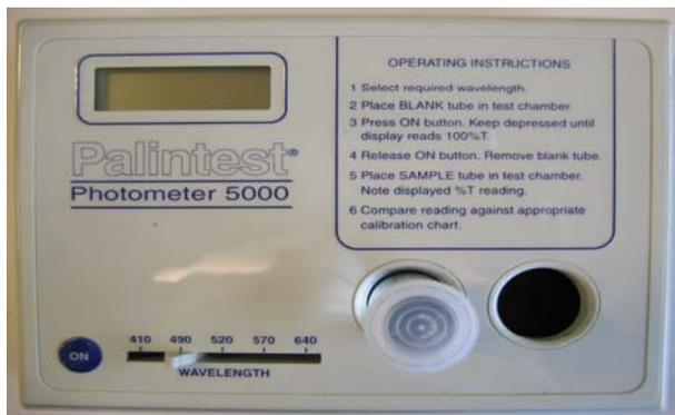
Photo 4: Example of a Photometer manufactured by Palintest.
