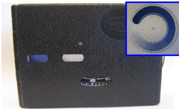
**Photo 2: Example of a Colour Wheel Comparator manufactured by HACH**
