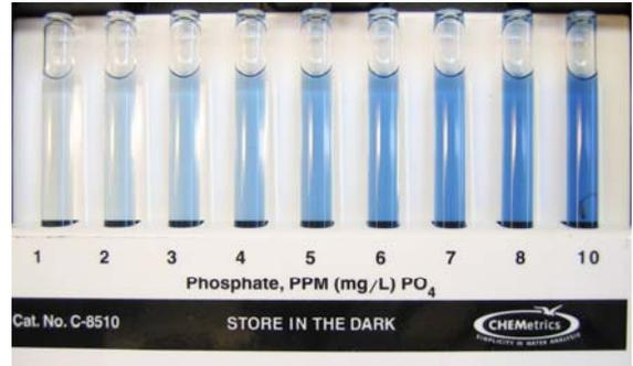
**Photo 3: Example of a Set of Liquid Colour Standards manufactured by CHEMetrics**
