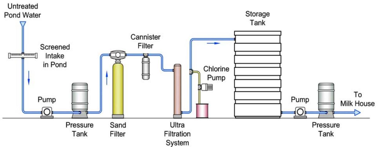
**Figure 1: Typical Treatment Train for Ultra-Filtration System**
