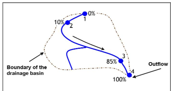
Figure 1 : Determination of the average longitudinal slope of a drainage basin
