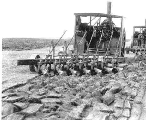
Figure 5: Two Marshall gas tractors 8 (35-70 HP) breaking sod on the Canadian Wheatlands Company Limited holdings near Suffield, in 1913 (Glenbow Archives, NA-587-8).
