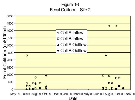
There was little water flow through the system in 1999 due to low runoff volumes from the feedlot. The long hydraulic retention time of the system, including the holding pond, is again evident as some of the data shows very low concentrations of contaminants in the wetland inflow. Comments on selected parameters is presented below.
