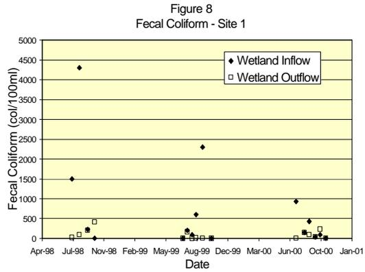
There was little water flow through the system in 1998 and 1999 since these were very dry years and there was little runoff from the feedlot. Some of the data, such as the wetland inflow ammonia concentration, reflect a very long hydraulic retention time within the holding pond, especially in 1999, resulting in almost complete nitrification. Comments on selected parameters are presented below.
